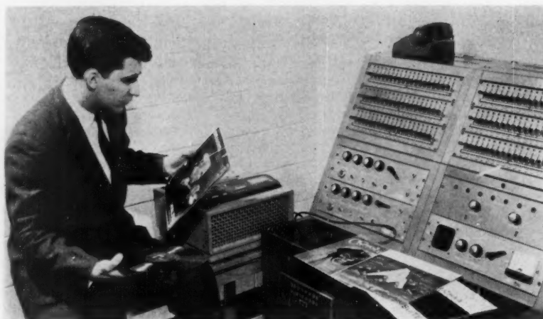
The author prepares his morning program of "Before-Home-Room Music" using the Bogen-Presto Console Control Center of the Public Address System.
